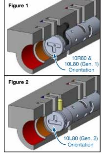
**For 10L80 (Gen. 2) Valve Body Orientation:** Carefully insert Sonnax O-ringed end plug into the bore just far enough to reinstall the OE retainer. Use a flat-head screw driver to rotate the end plug so the T-groove resembles an upsidedown capitol "T" (**Figure 2**).
