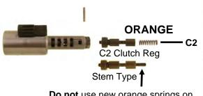
Do not use new orange springs on C2 or C3 Clutch Reg if your valve has a stem located here.
