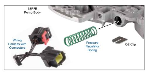
NOTE: This kit is not recommended for use with transmission tuning mods. If you are unsure of the vehicle's programming, use a scan tool to verify transmission line pressure meets stock levels (Drive at idle = 60 psi, Drive under heavy load = 160 psi). If desired line pressure values are greater than this, the system most likely has aftermarket tuning mods to the transmission pressure.
