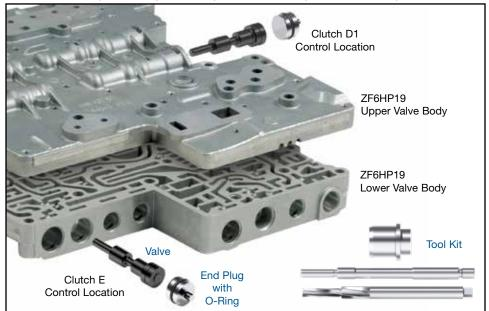
CAUTION: Sonnax kit is NOT compatible with '12-later 6R80 applications that contain an OE "D1" valve with two equal diameter spools (Figure 1). Valve bodies with separator plate AL3P-7Z490-BA contain this incompatible OE valve. Note, however, this Sonnax kit can still be used in "E" bore for these applications.
