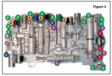
Lower Valve Body, Case Removal - Bolt Locations
