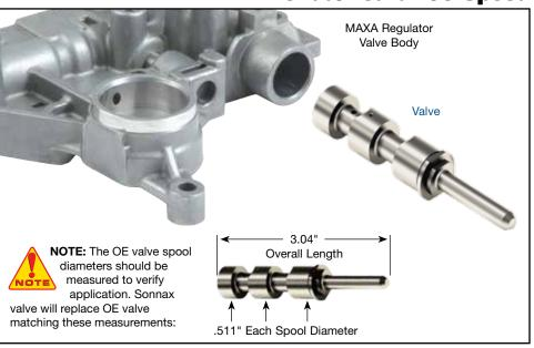
**CAUTION:** The main pressure regulator valve is secured with relatively high spring force. Exercise caution when removing the retaining bolt and regulator spring cap, as these parts can eject from the valve body with strong force and high speed, potentially causing injury or property damage.
